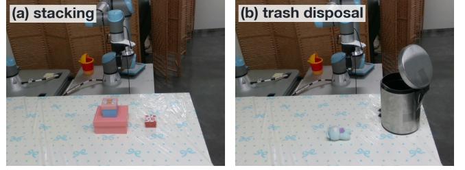
Fig. 3. Physical evaluation tasks on the UR5e. (a) Box stacking. (b) Long-range transport into a trash bin.
